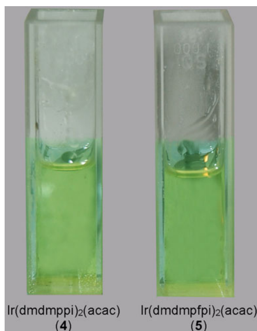
Fig. 9 Solution colour of the photoluminescence for complexes 4 and 5
